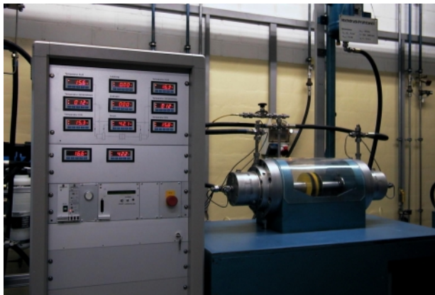
Picture 1: Mechanical Seal High Pressure Test Rig
